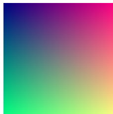
Figure 1: setup_ok.ppm , enlarged: r = 4x , g = 4y , b = 128 . Red grows rightward ( x ), green grows downward ( y ).
